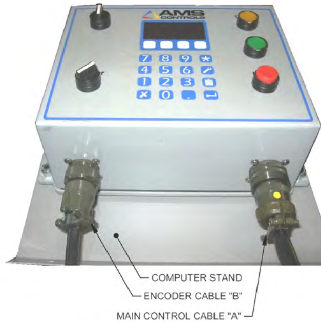
Figure 36: AMS Box With Cables
